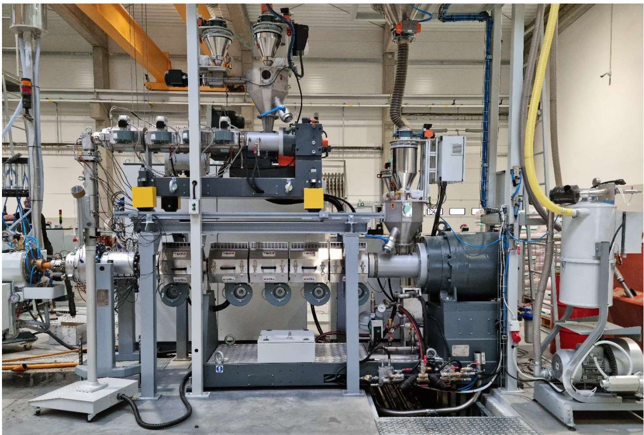
Figure 1 - A multilayer extrusion line with gearless extruder and piggyback co-extruder for external layer.
